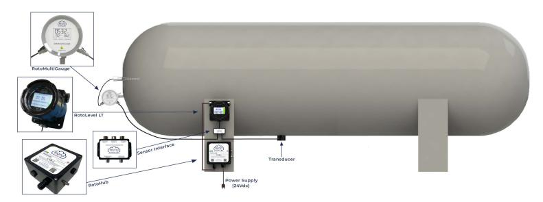
The RotoMultiGauge also forms part of an innovative high technology solution for controlling the inventory of a storage tank. When integrated with our ultrasonic level measurement device (RotoLevel LT) and telemetry device (RotoHub), the user is able to manage and control their tank inventory via our secure online DataPortal. More details on Page 6.
